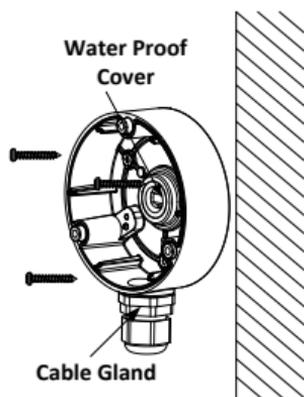
Figure 2-7 Fix the Junction Box on the Wall
