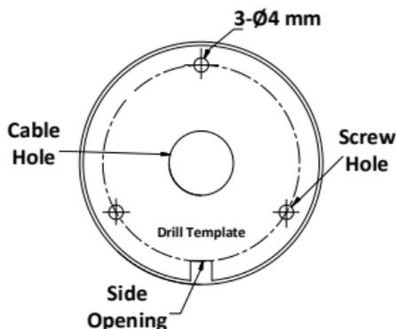
Figure 2-2 The Drill Template
