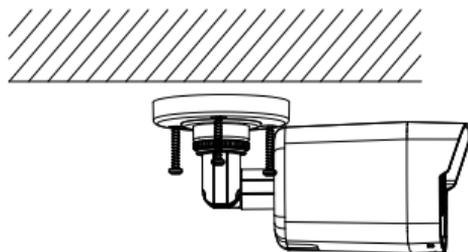
Figure 2-3 Fix the Camera on the Ceiling
