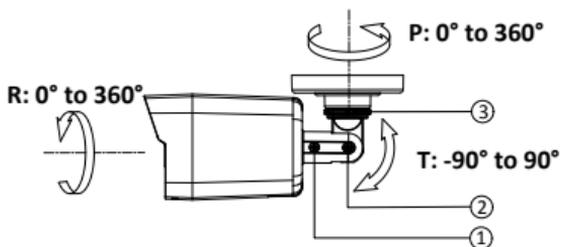
Figure 2-4 3-axis Adjustment
