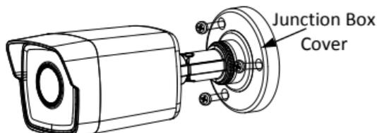
Figure 2-6 Fix the Camera on Junction Box's Cover
