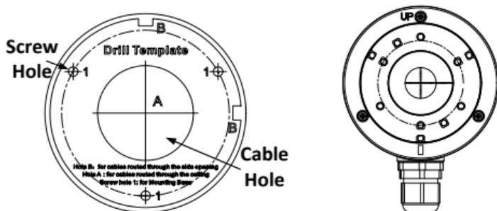
Figure 2-5 The Drill Template
