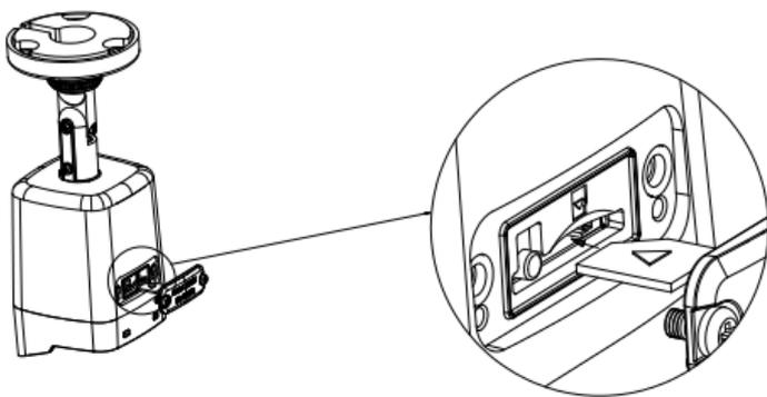
Figure 2-1 Unscrew the Cover and Insert Memory Card
