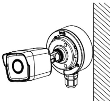
Figure 2-8 Combine Junction Box's Cover with its Body
